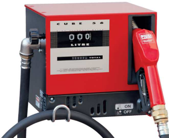
CUBE 56 (pump inside) Flow rate 15 gpm Accuracy +/- 1% Inlet: 1" BSP / 1" NPT Fluids: Diesel
